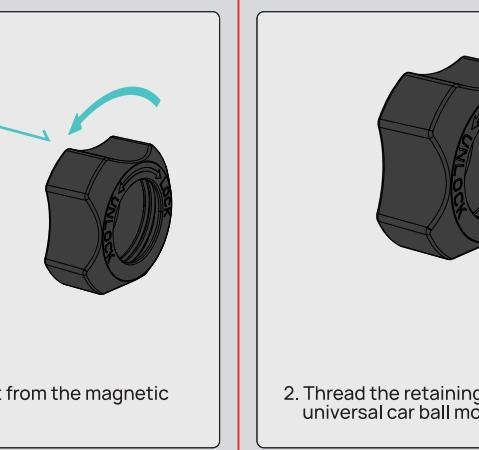
1. Remove the retaining nut from the magnetic wireless charger
