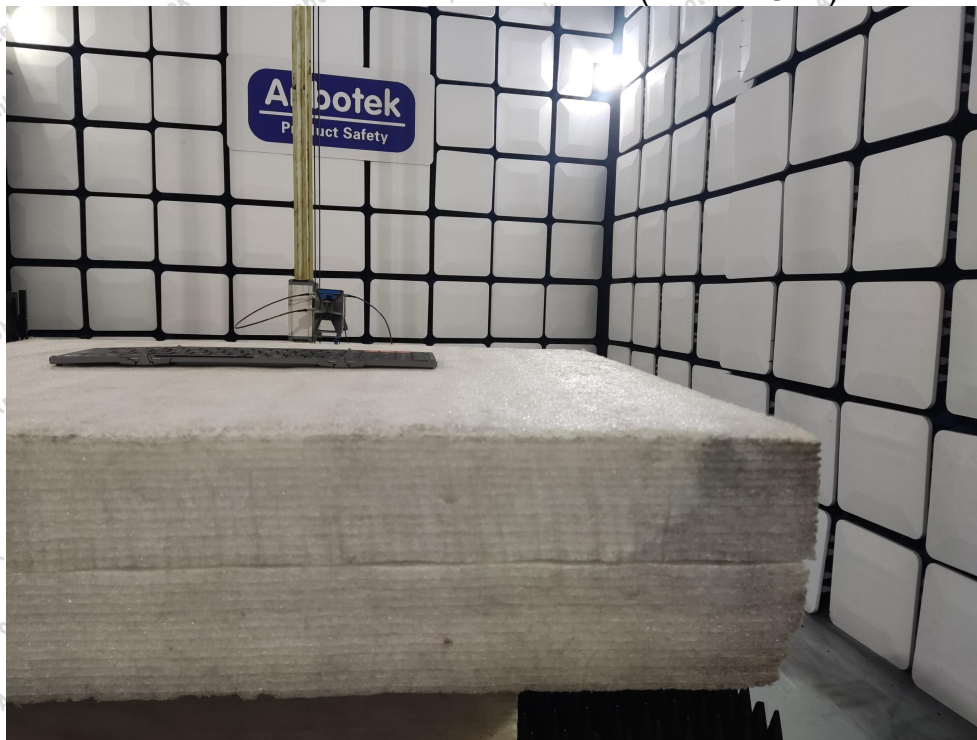
Photo of Radiation Emission Test (above 1GHz)
