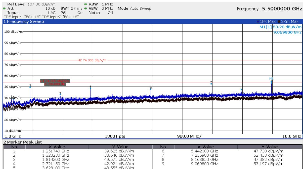
Limit according to FCC Part 15C, Section 15.209:
