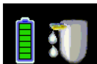
Figure 2-6: Good quality of charging the alfapump®
