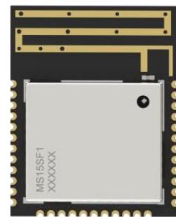
MS15SF1 is a multi-protocol, high-performance, cost-effective wireless WiFi 6+BLE5.3 combo module based on ESP32-C6 SoC. The RISC-V single-core runs at a frequency of 160 MHz, with 320 KB+4MB FLASH program space, 512KB+16KB RAM, integrated 2.4 GHz transceiver, LNA, and other powerful resources for 2.4GHz WiFi/BLE connections. It is compatible with the MS11SF11 module and can withstand voltages of up to 80M in actual high-interference conditions. MS15SF1 is compatible with the MS11SF11 module.
