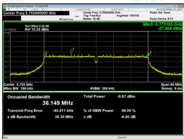
(802.11ac40) PSD plot on channel 151
