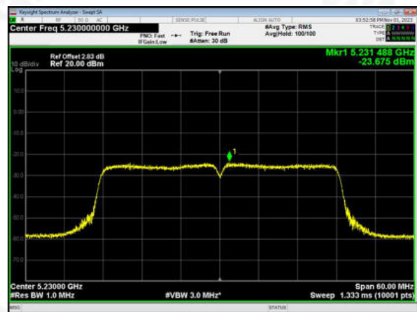
(802.11ac40) PSD plot on channel 46
