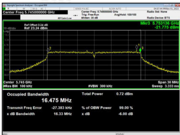
(802.11a) 6dB Bandwidth plot on channel 149
