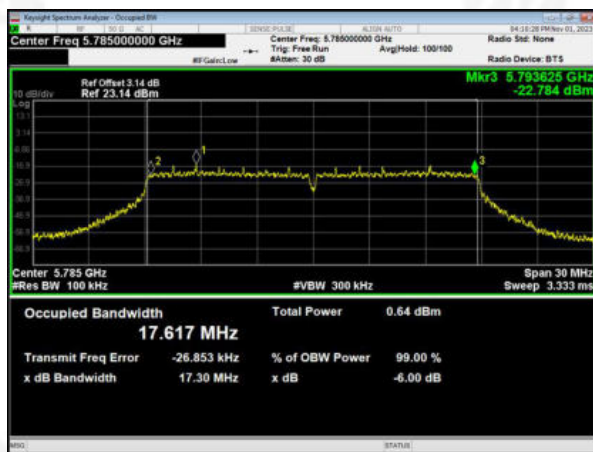
(802.11ac20) 6dB Bandwidth plot on channel 165
