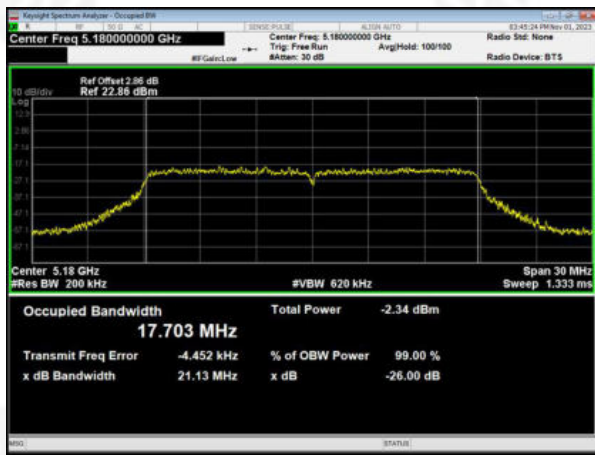
(802.11 ac20) 26dB Bandwidth plot on channel 40
