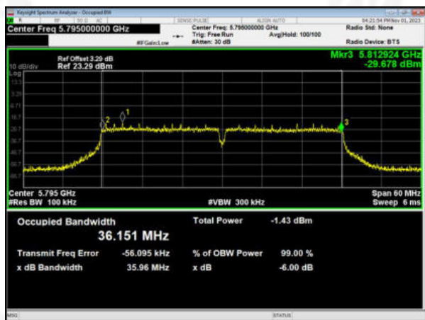
(802.11ac40) PSD plot on channel 159
