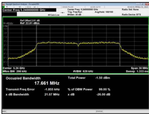
(802.11 ac20) 26dB Bandwidth plot on channel 48
