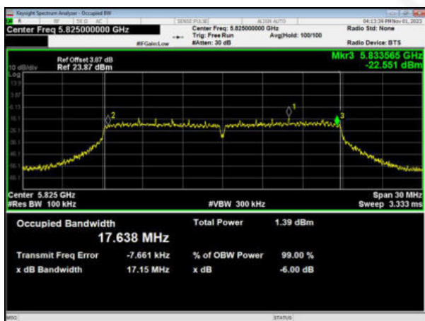
(802.11n20) 6dB Bandwidth plot on channel 165
