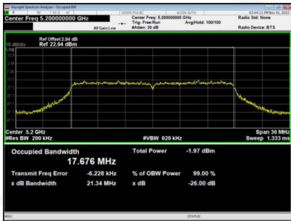
(802.11 ac20) 26dB Bandwidth plot on channel 48
