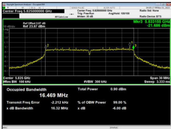
(802.11a) 6dB Bandwidth plot on channel 165
