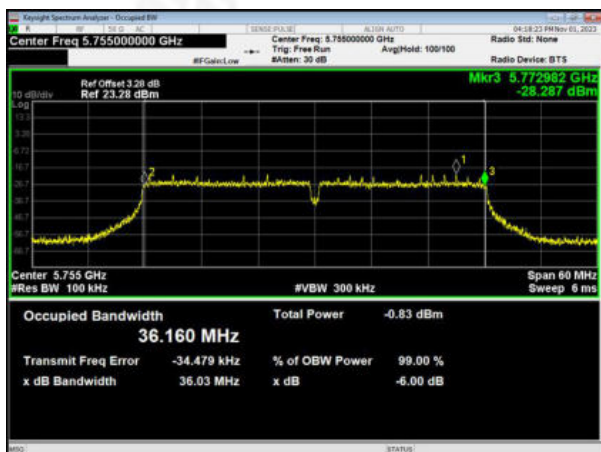
(802.11n40) PSD plot on channel 151
