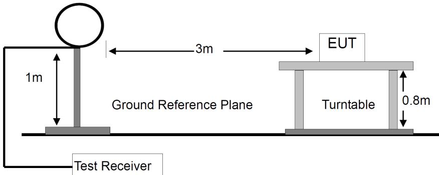
For Radiated Emission 30-1000MHz
