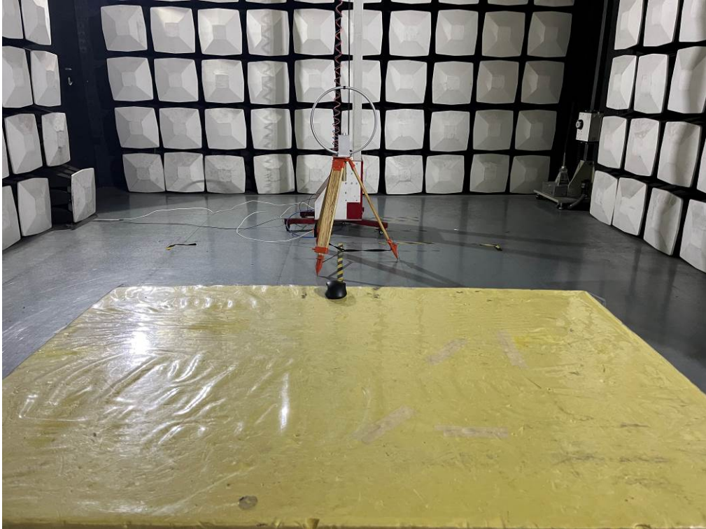
Radiated emission (30-1000MHz)
