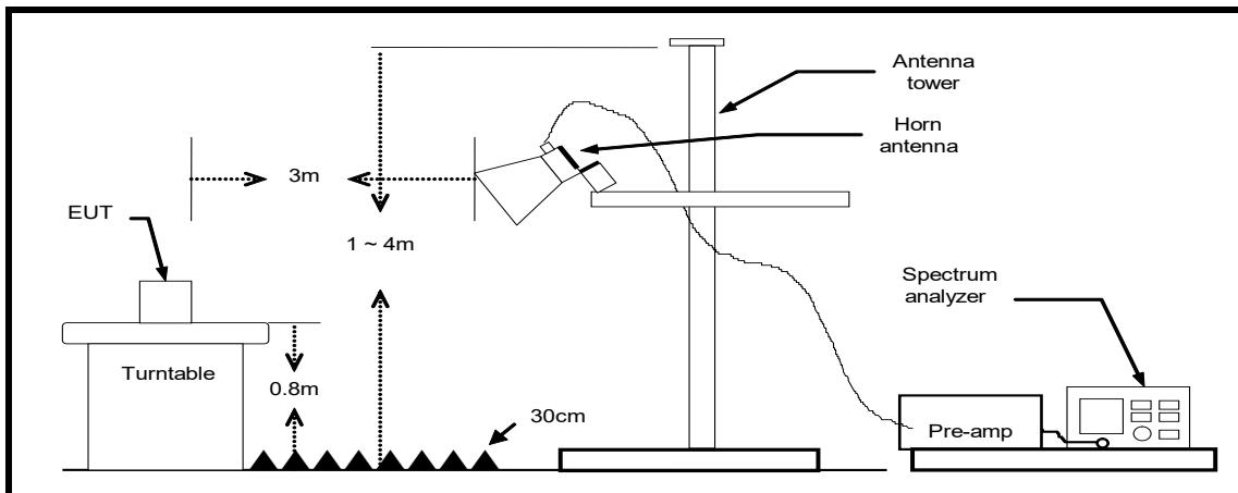
Test arrangement for radiated emissions of tabletop equipment.
