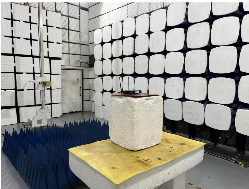
Above 1GHz- Transmitter unwanted emissions
