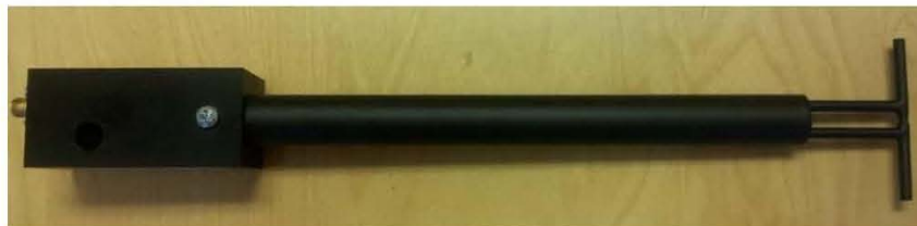
Figure 1 – MVG COMOSAR Validation Dipole
