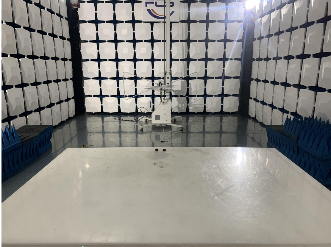
Above 1GHz for radiated emission test setup
