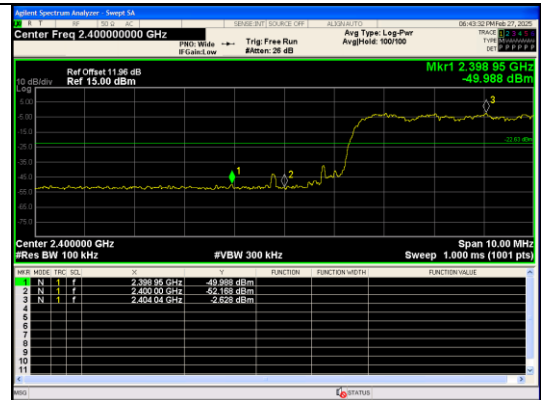
Out Of Band Emission(Left) \pi/4 DQPSK_2-DH5_Channel Hopping
