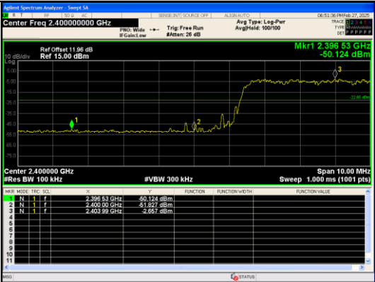
Out Of Band Emission(Left) 8DPSK_3-DH5_Channel Hopping
