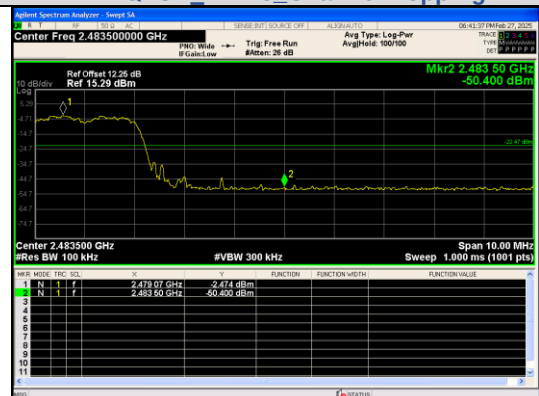
Out of Band Emission(Right) \pi/4 DQPSK_2-DH5_Channel Hopping
