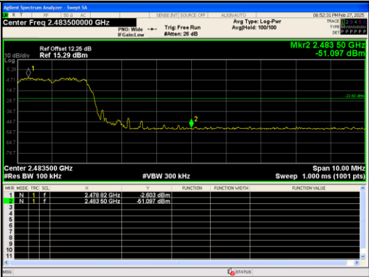
Out Of Band Emission(Right) 8DPSK_3-DH5_Channel Hopping
