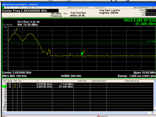
Out of Band Emission(Right) GFSK_DH5_Channel Hopping
