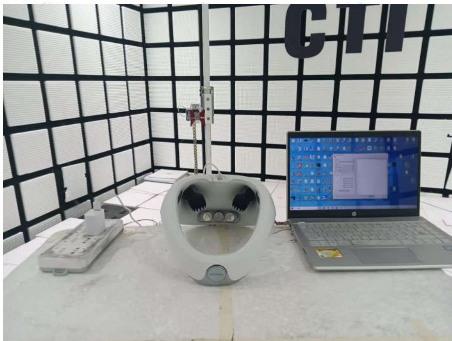
Radiated spurious emission Test Setup-2(Above 1GHz)
