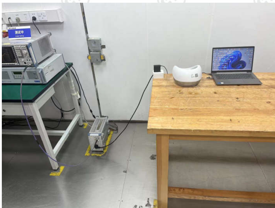
Conducted Emissions Test Setup
