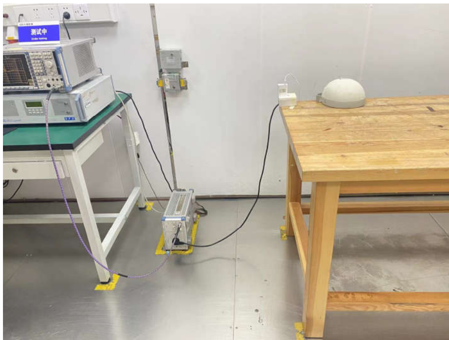
Conducted Emissions Test Setup
