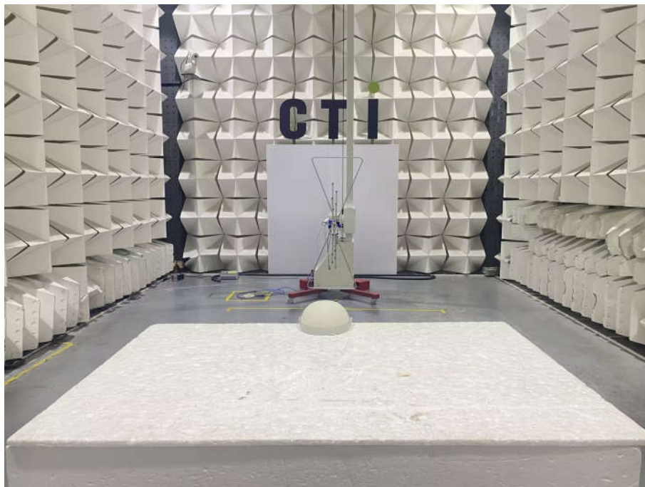
Radiated spurious emission Test Setup-1(Below 1GHz)
