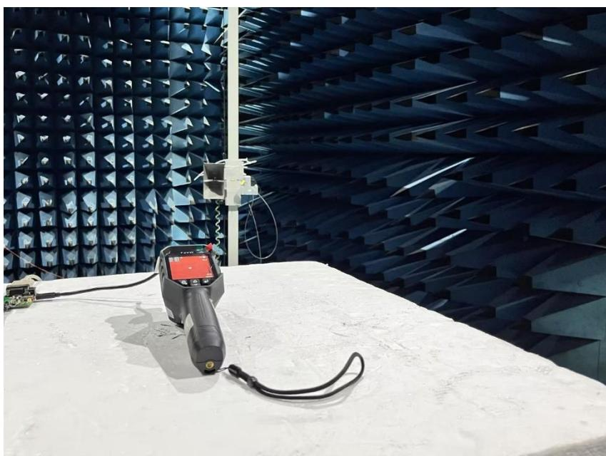
**Radiated Test Below 1GHz**
