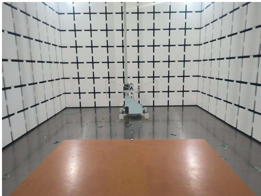
**Radiated Emission Test View 2 (Right earphone)**
