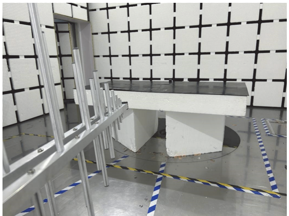
Radiation Emission Test Setup (30MHz to 1GHz)
