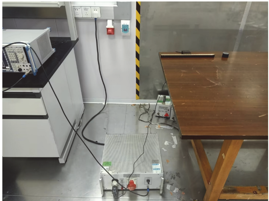
Conducted Emission Test Setup
