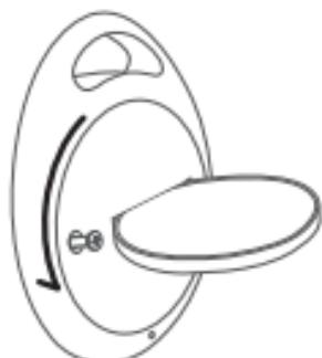
2. Replace the battery with a new CR2032 type battery, placing the battery positive side up;
