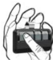
**Example:** If learn button of opener is **red**, press the button **three** times.
