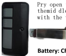
Pry open the case first in the middle, then at each side with the visor clip.
