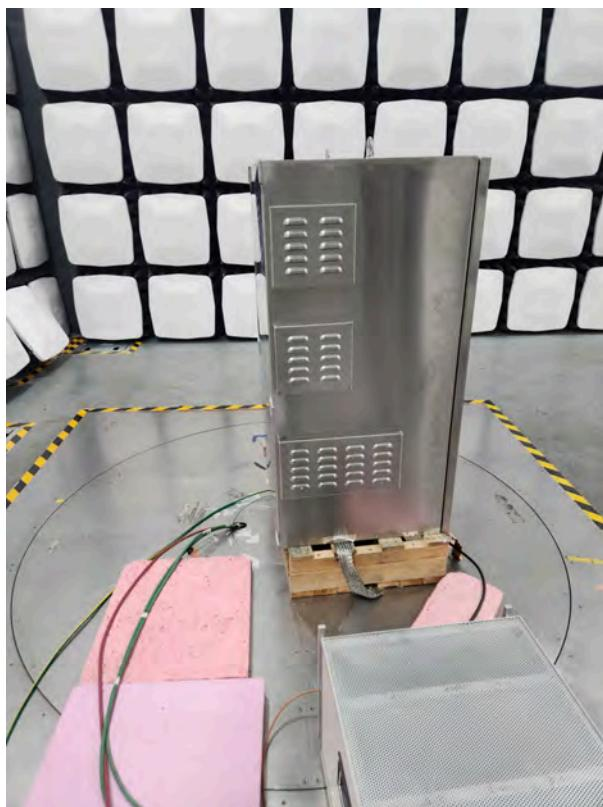
**Radiated Emission (30 MHz ~ 1 000 MHz)**
