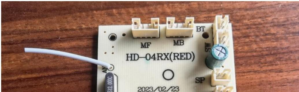
Note: The 2.4G antenna specification is a 12 core outer diameter 1.3mm bare copper wire wire, white, with a length of 35mm. The wire end is peeled off with 3MM tin. Complies with environmental standards: EU EN71 (19E), ROHS, PAHS, 6P-16P, European and American CPSIA, HR4040.
