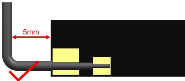
FIGURE 5.2.1 RECOMMENDED CABLE BENDING RANGE
