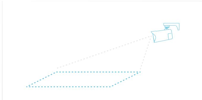
Choose a suitable location to mount the camera (ensure the camera's view covers the pool area without blind spots and avoid pointing directly at the sun). Using the provided template, mark and drill two holes, mount the bracket, and slide the camera into the bracket.
