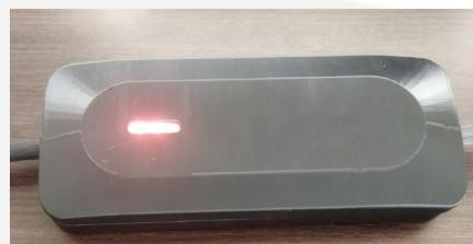
If the charger turns red when it is turned on, it means that the electrical network is not in a condition to be able to carry out the vehicle charging process. This can be due to:
