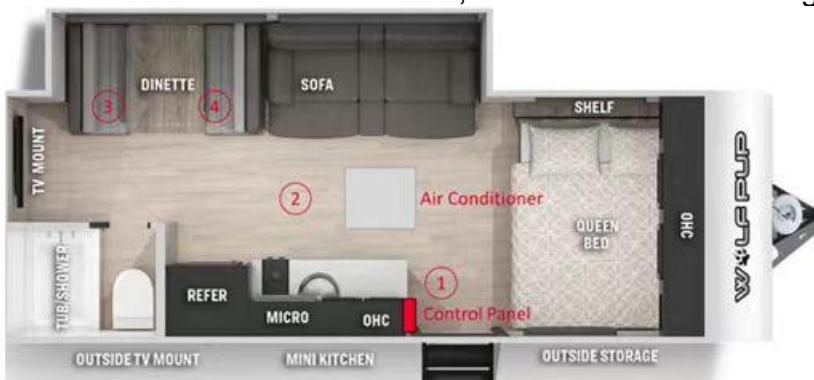
The module is installed in the WFCO smart power control system position 1 in
