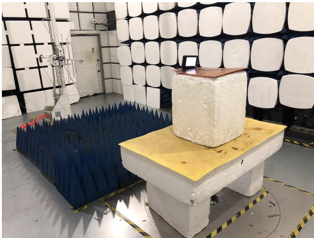
Radiated Emissions Measurement (Below 1GHz)
