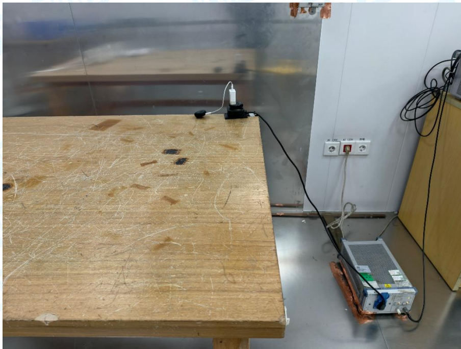
Photo of Setup for Conducted Emission
