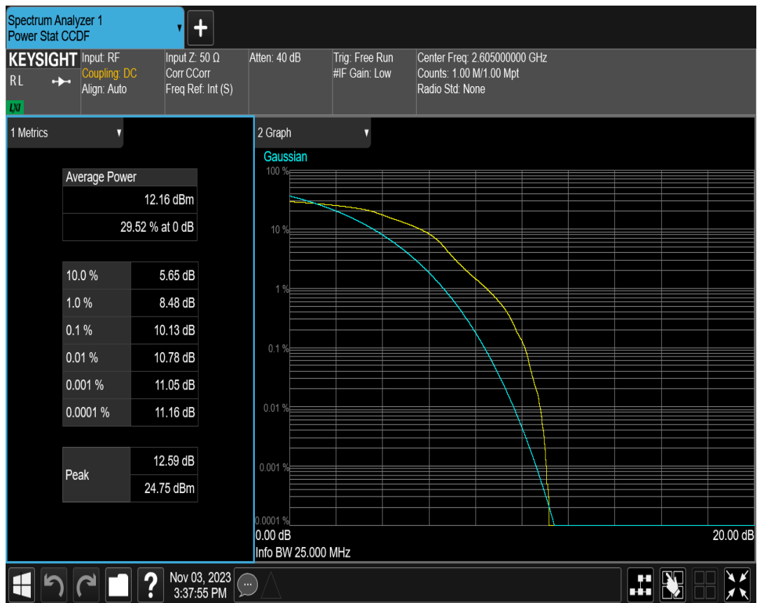
Band41(2555-2655) QAM16 BW=20MHz Channel=40740 RB Size=1 Position=#0
