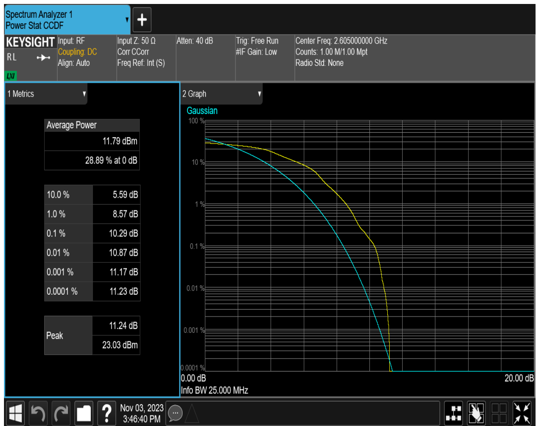
Band41(2555-2655) QAM16 BW=5MHz Channel=40740 RB Size=1 Position=#0
