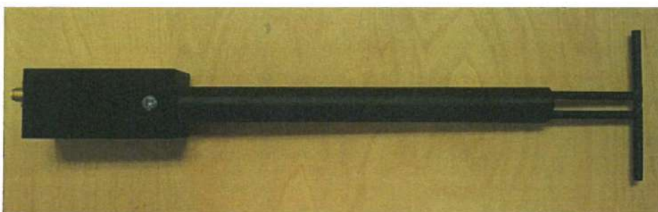
Figure 1 – MVG COMOSAR Validation Dipole
