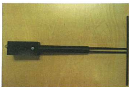
Figure 1 – MVG COMOSAR Validation Dipole
