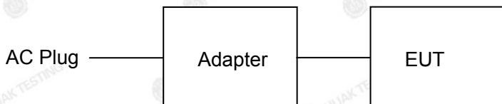
Operation of EUT during Above1GHz Radiation testing:
