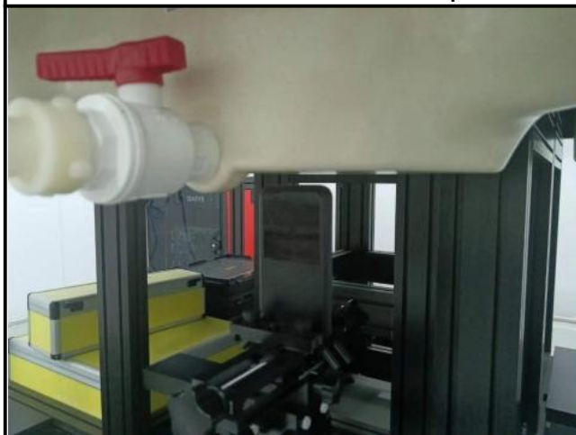
Top Side of EUT with 1.0 cm Gap
