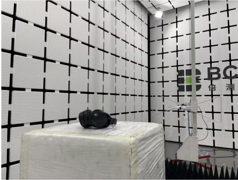
Spurious Emission Test Setup (Above 1GHz)
