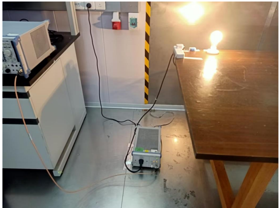
Conducted Emission Test Setup
