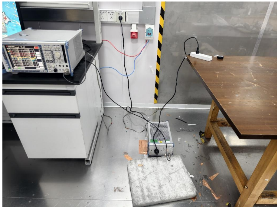
Conducted Emission Test Setup
