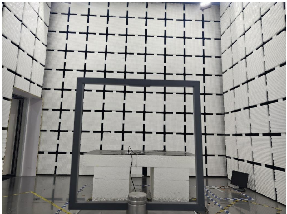
Radiation Emission Test Setup (Below 30MHz)
