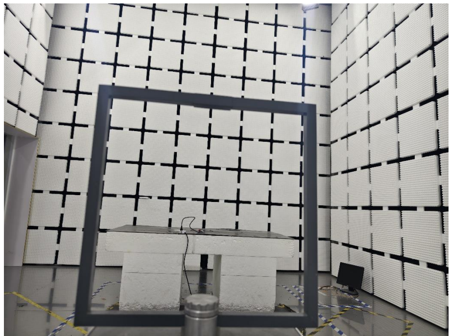
Radiation Emission Test Setup (Below 30MHz)
