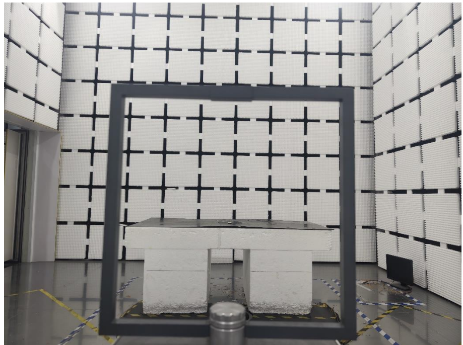
Radiation Emission Test Setup (Below 30MHz)
