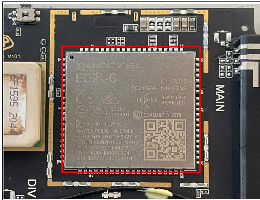
**Top view of WWAN Module without Shielding**
