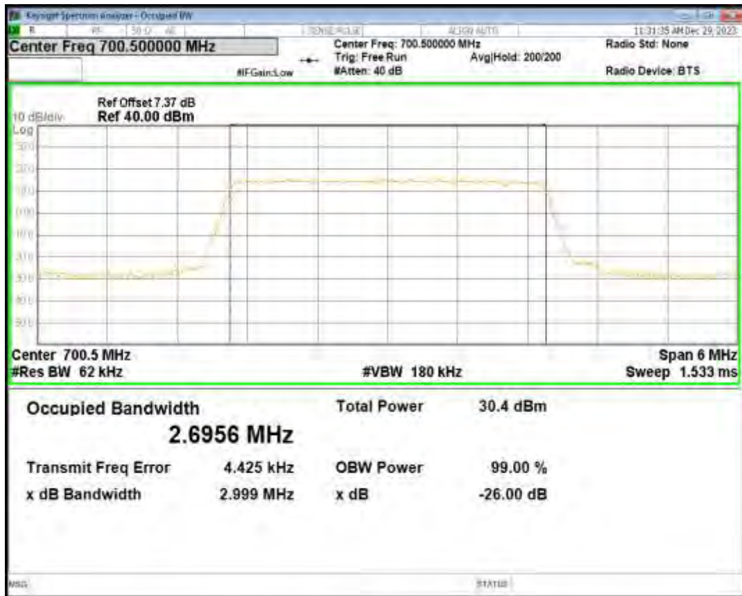
Band12 QPSK BW=3MHz Channel=23095 RB Size=15 Position=#0
