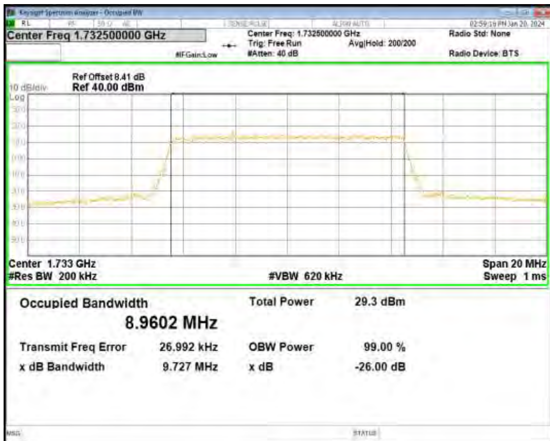
Band4 QPSK BW=15MHz Channel=20325 RB Size=75 Position=#0
