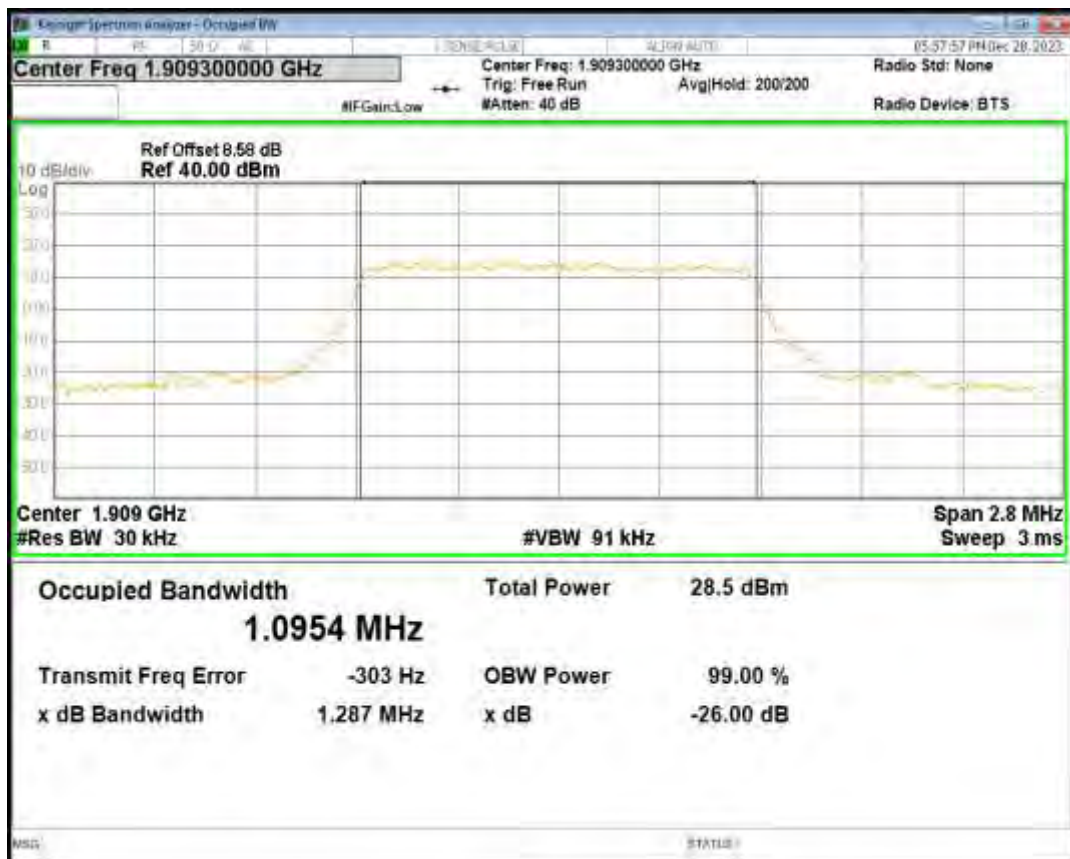
Band2 16QAM BW=10MHz Channel=18650 RB Size=50 Position=#0
