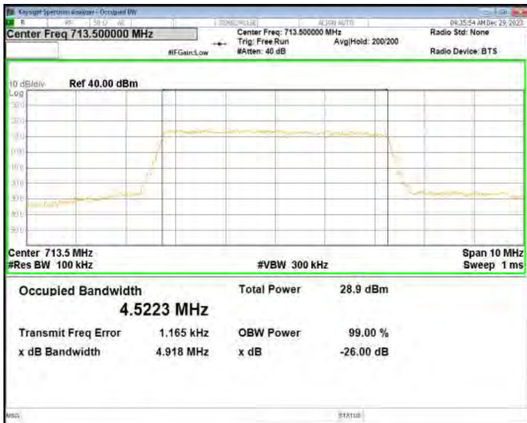
Band17 QPSK BW=10MHz Channel=23780 RB Size=50 Position=#0
