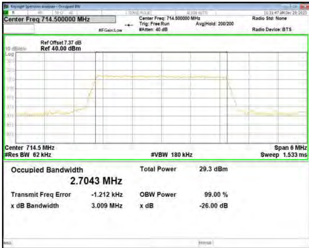
Band12 16QAM BW=5MHz Channel=23035 RB Size=25 Position=#0
