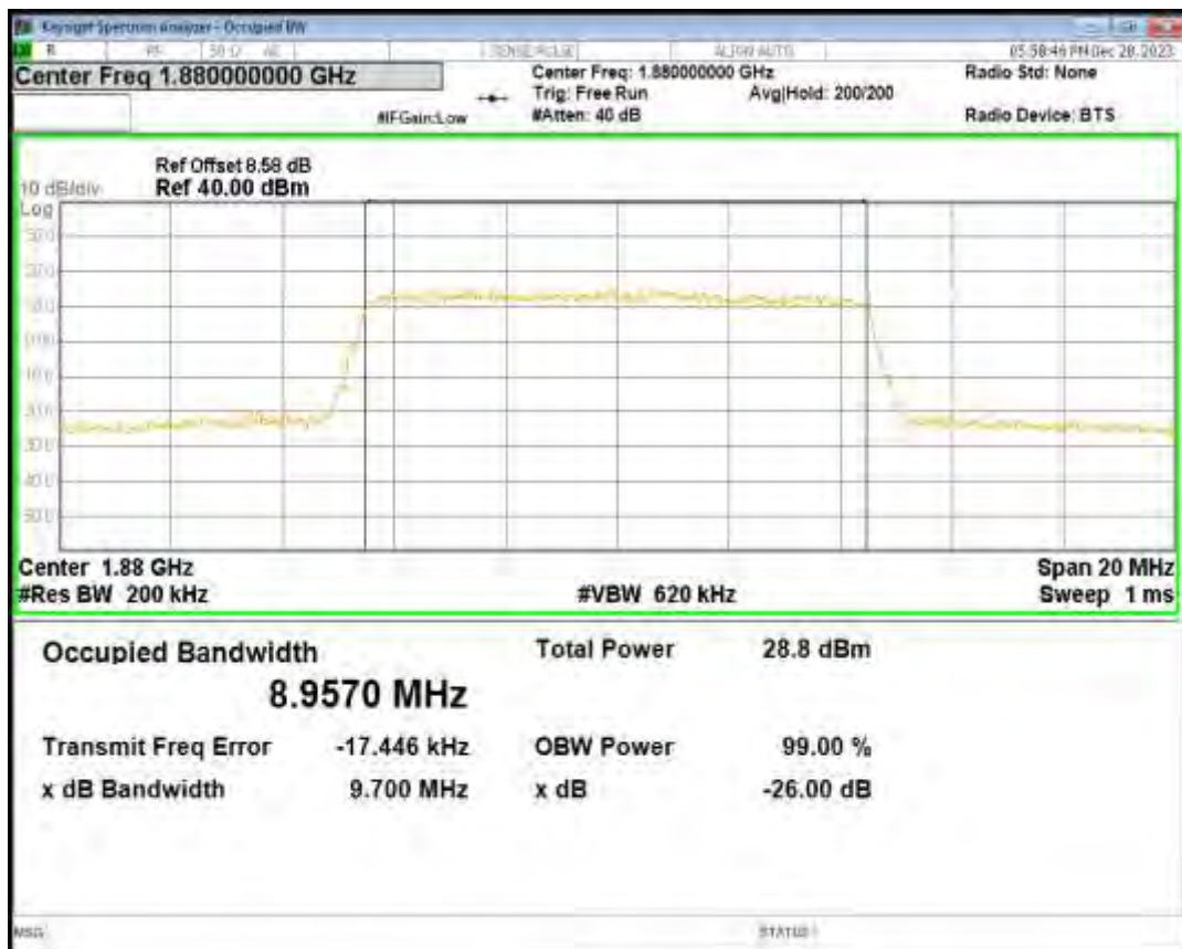
Band2 16QAM BW=10MHz Channel=19150 RB Size=50 Position=#0
