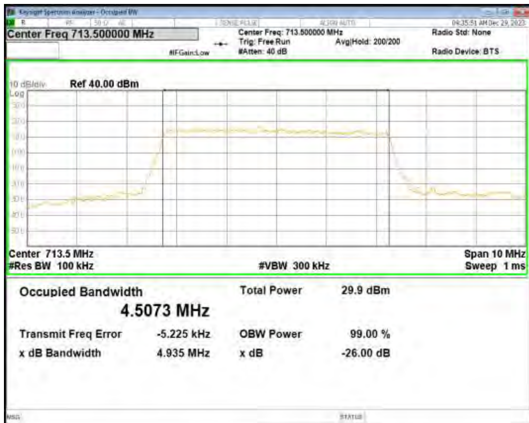
Band2 16QAM BW=1.4MHz Channel=18607 RB Size=6 Position=#0
