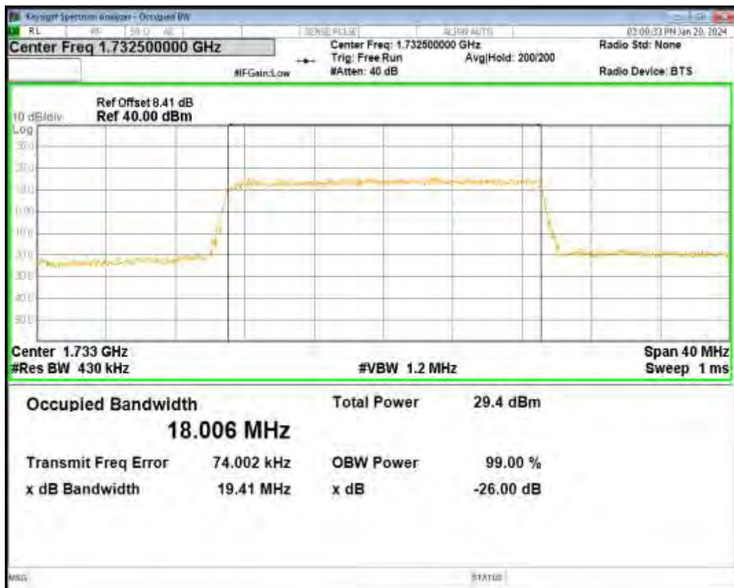
Band4 QPSK BW=20MHz Channel=20300 RB Size=100 Position=#0
