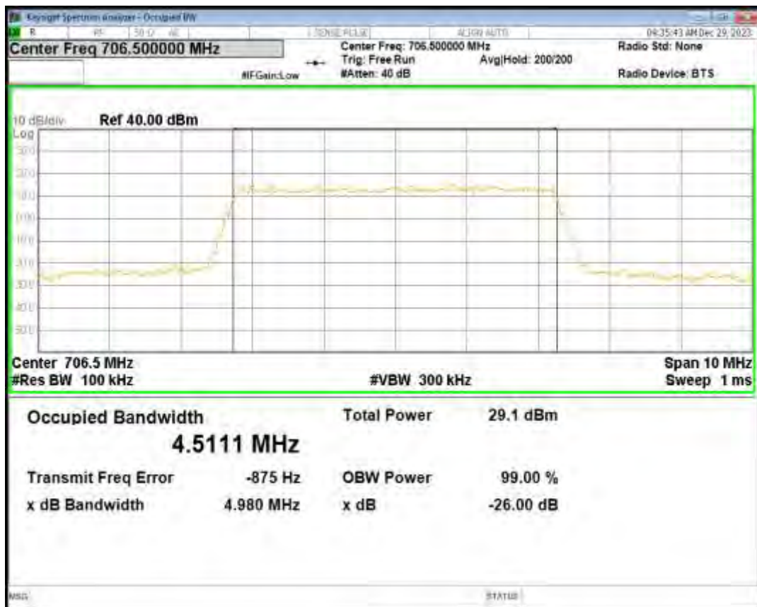
Band17 16QAM BW=5MHz Channel=23790 RB Size=25 Position=#0
