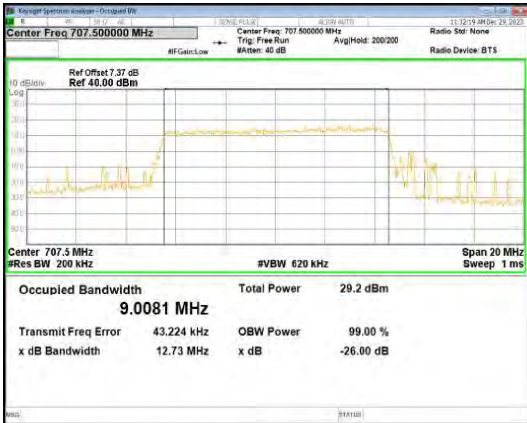
Band12 QPSK BW=10MHz Channel=23130 RB Size=50 Position=#0
