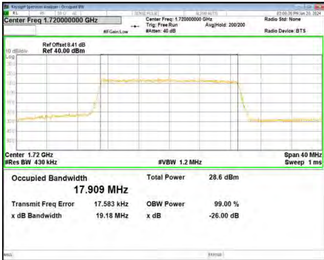
Band4 16QAM BW=20MHz Channel=20175 RB Size=100 Position=#0
