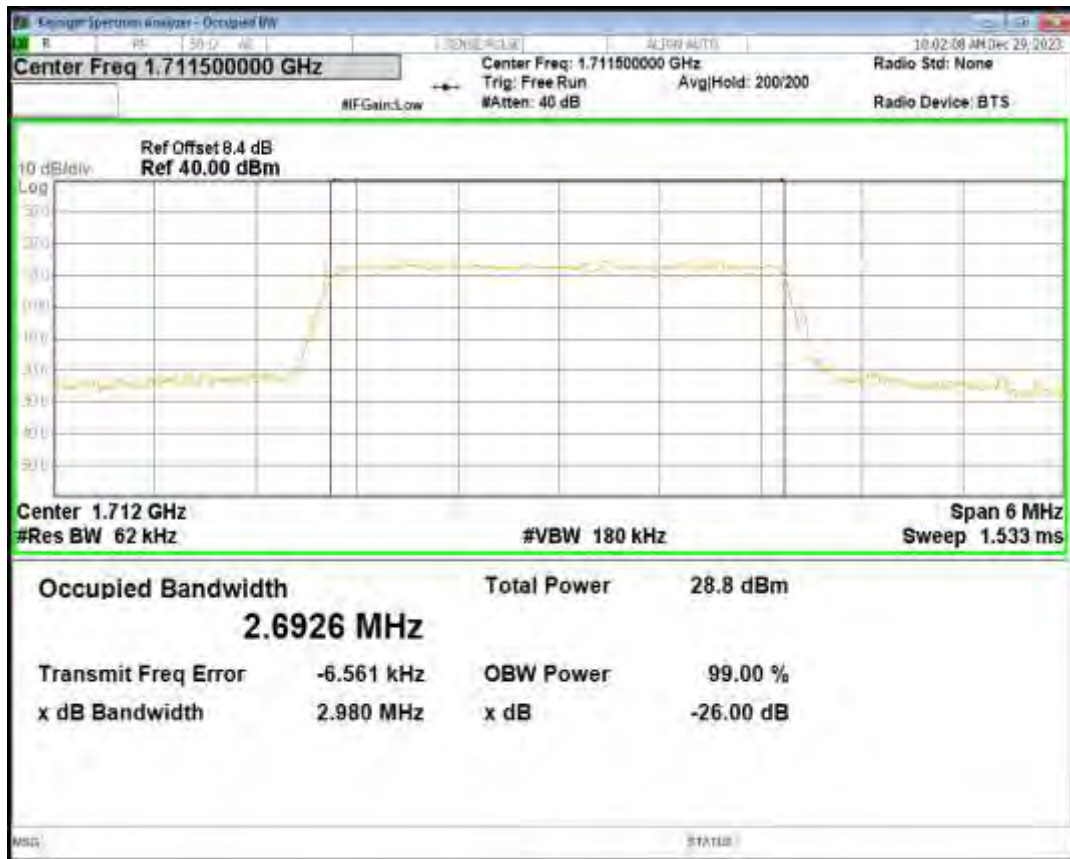
Band66 16QAM BW=3MHz Channel=132322 RB Size=15 Position=#0
