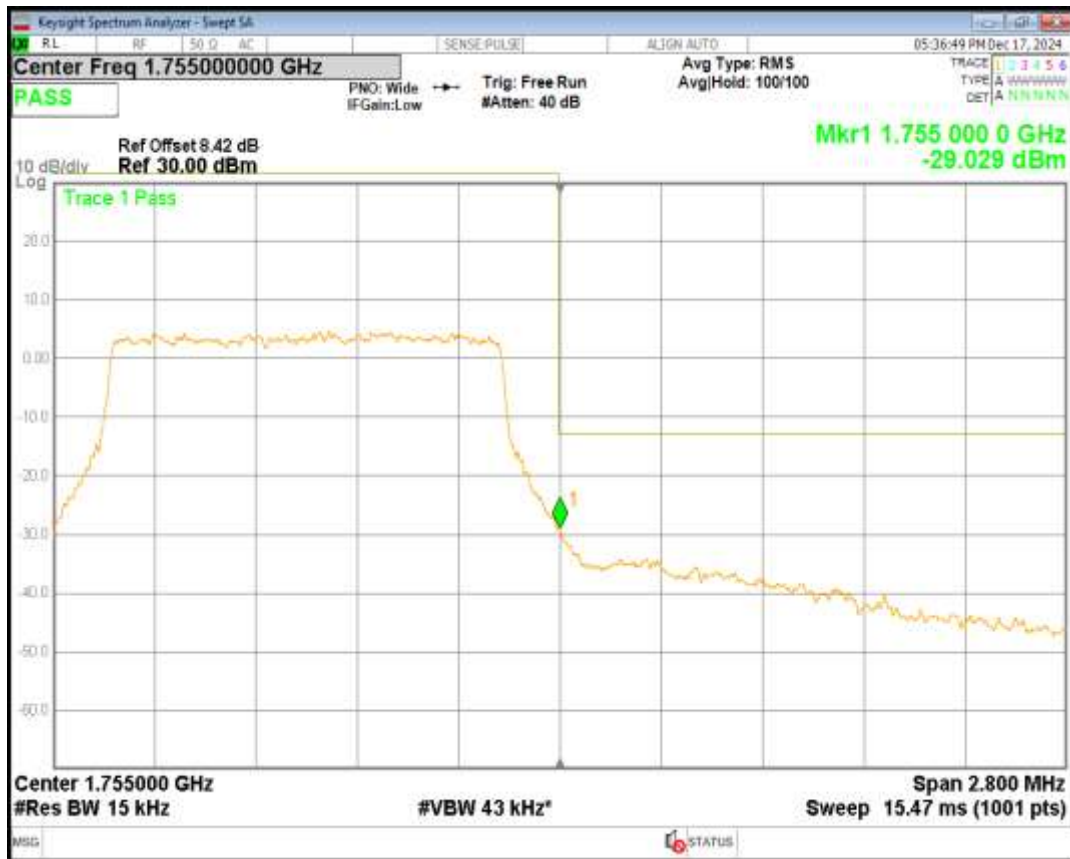
Band4 16QAM BW=10MHz Channel=20000 RB Size=50 Position=#0
