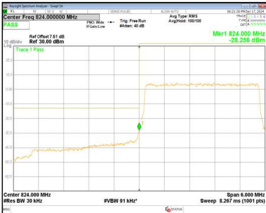
Band5 QPSK BW=3MHz Channel=20635 RB Size=15 Position=#0
