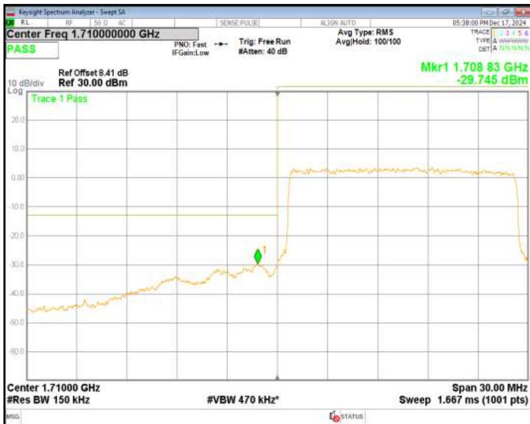
Band4 QPSK BW=10MHz Channel=20350 RB Size=50 Position=#0
