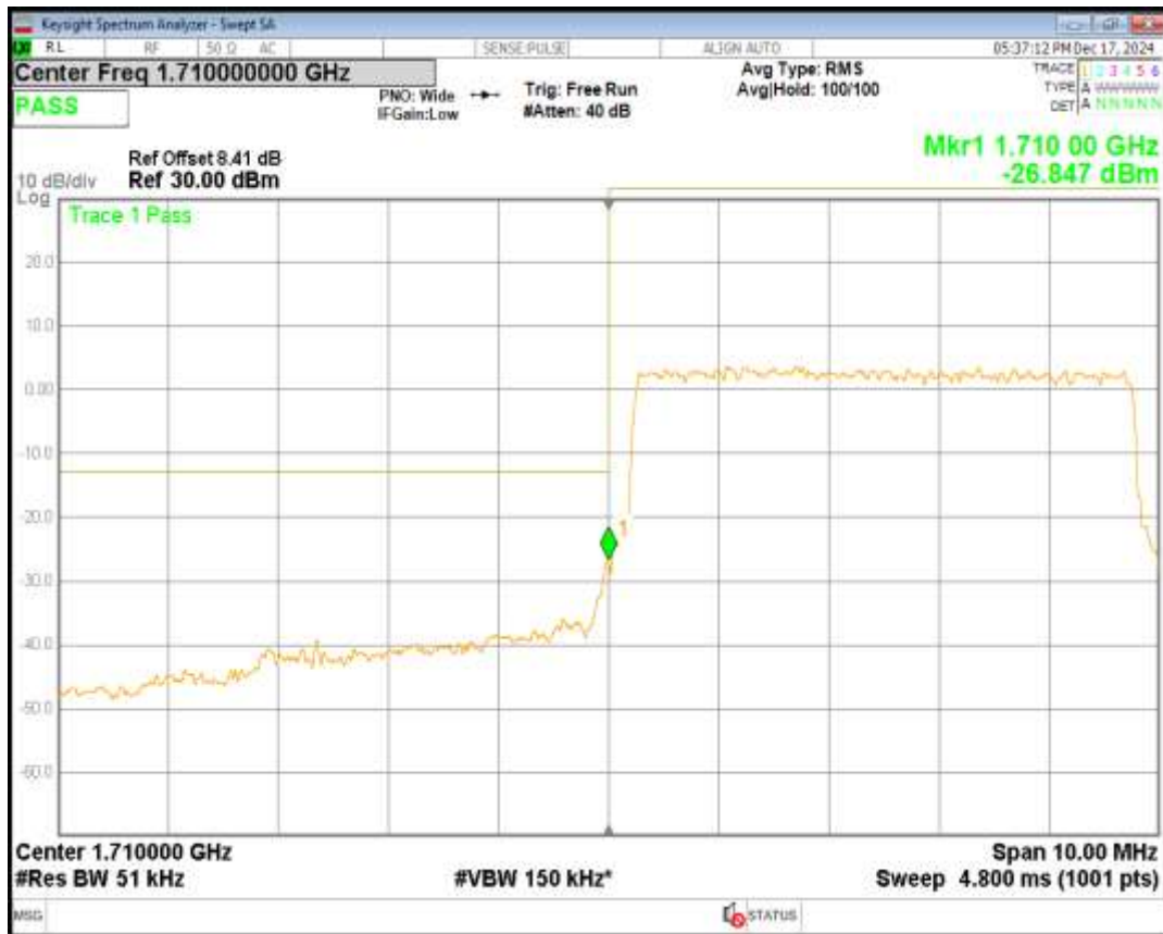
Band4 QPSK BW=20MHz Channel=20300 RB Size=100 Position=#0
