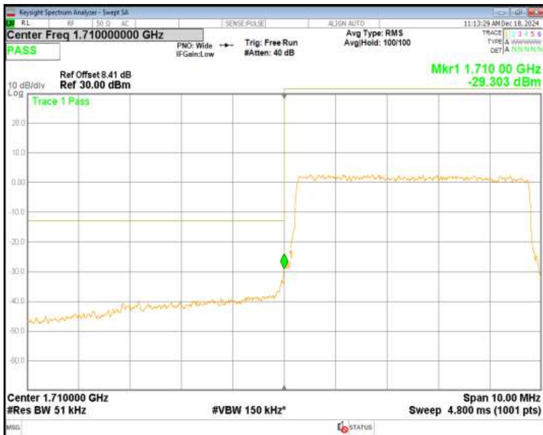
Band66 QPSK BW=20MHz Channel=132072 RB Size=100 Position=#0
