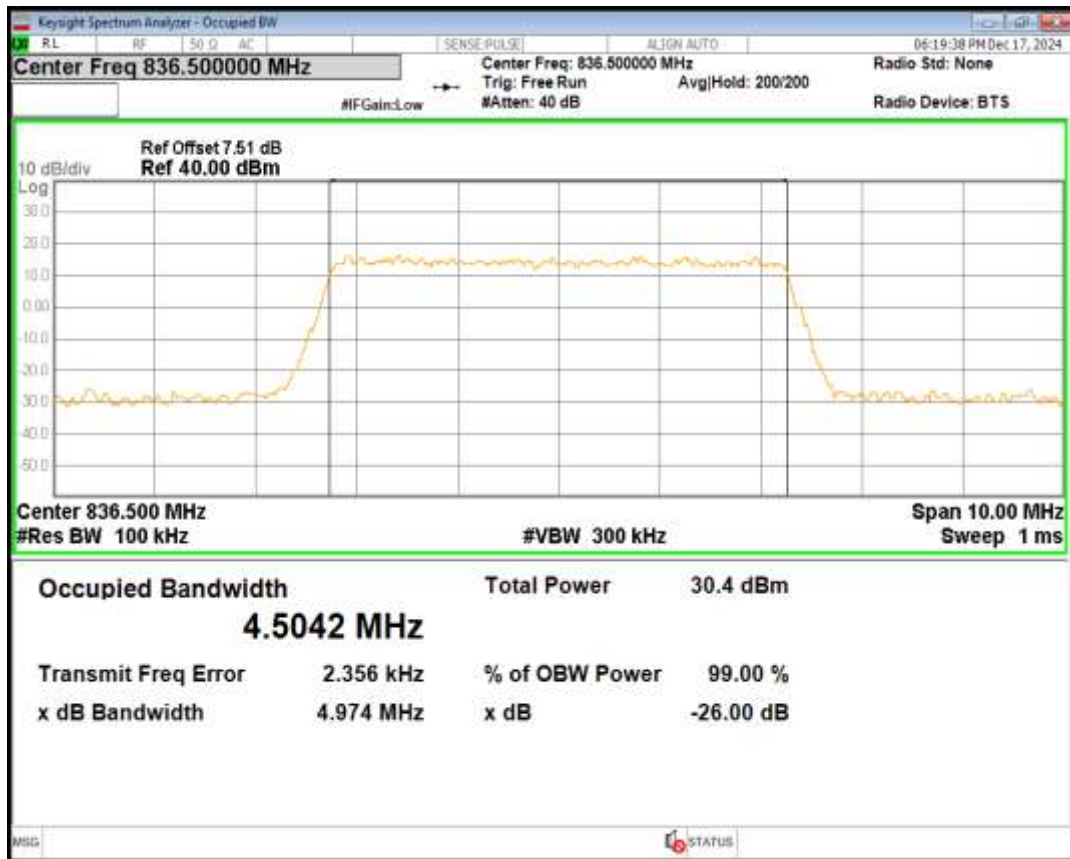
Band5 QPSK BW=5MHz Channel=20625 RB Size=25 Position=#0
