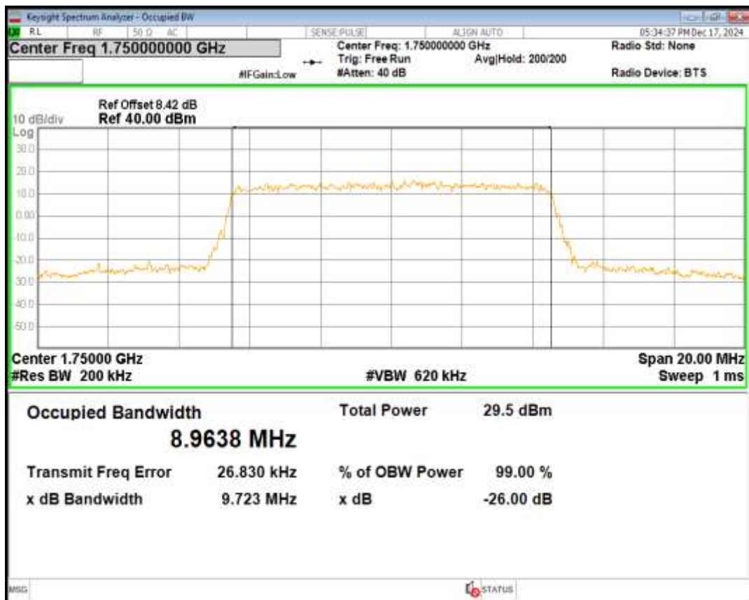
Band4 16QAM BW=3MHz Channel=20385 RB Size=15 Position=#0
