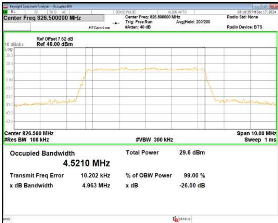
Band5 16QAM BW=3MHz Channel=20635 RB Size=15 Position=#0
