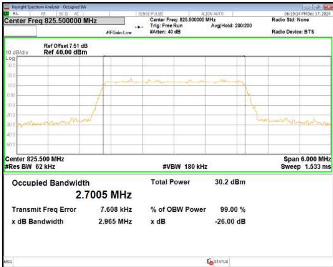
Band5 16QAM BW=3MHz Channel=20525 RB Size=15 Position=#0
