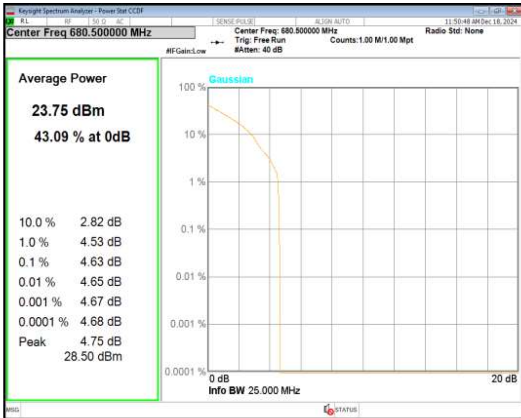
Band71 QPSK BW=15MHz Channel=133397 RB Size=1 Position=#0
