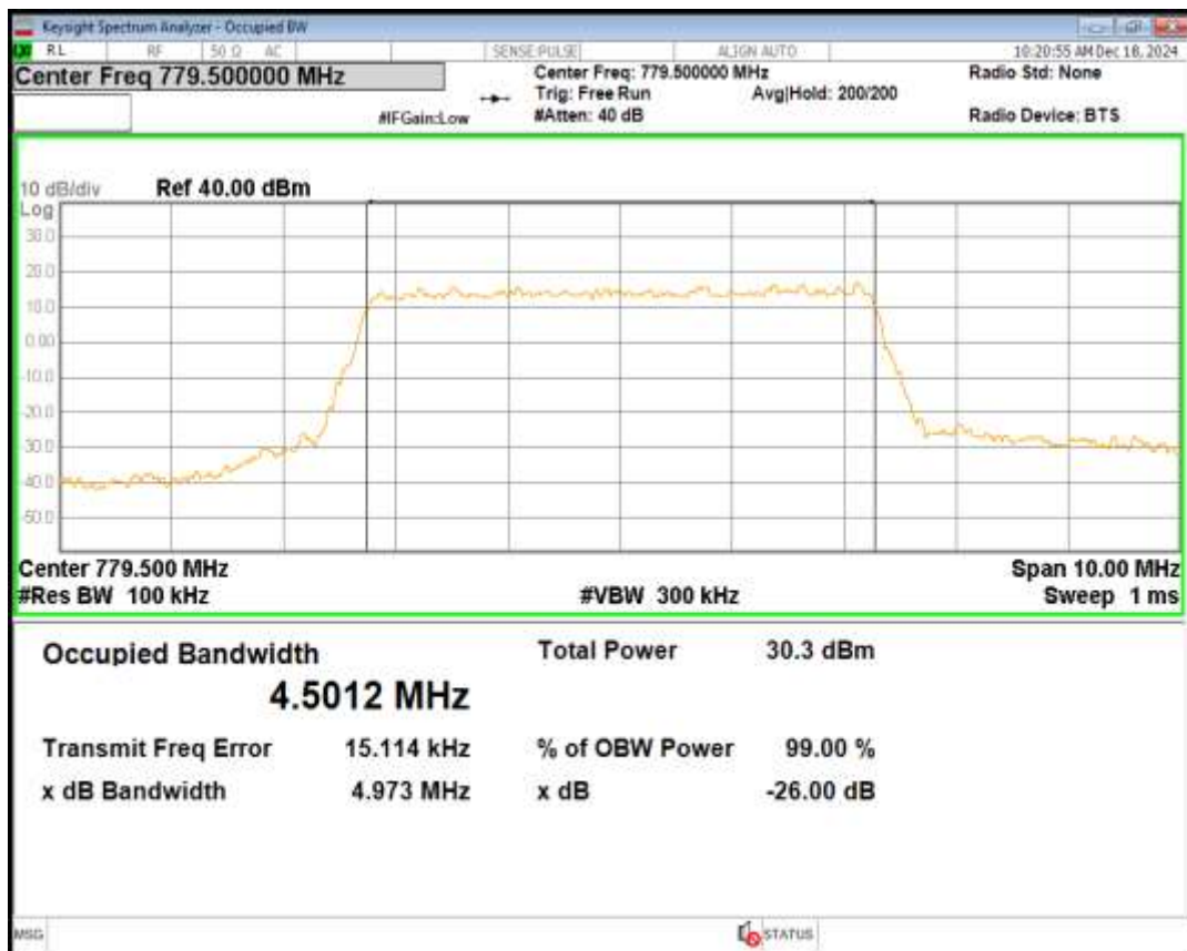
Band13 QPSK BW=5MHz Channel=23230 RB Size=25 Position=#0
