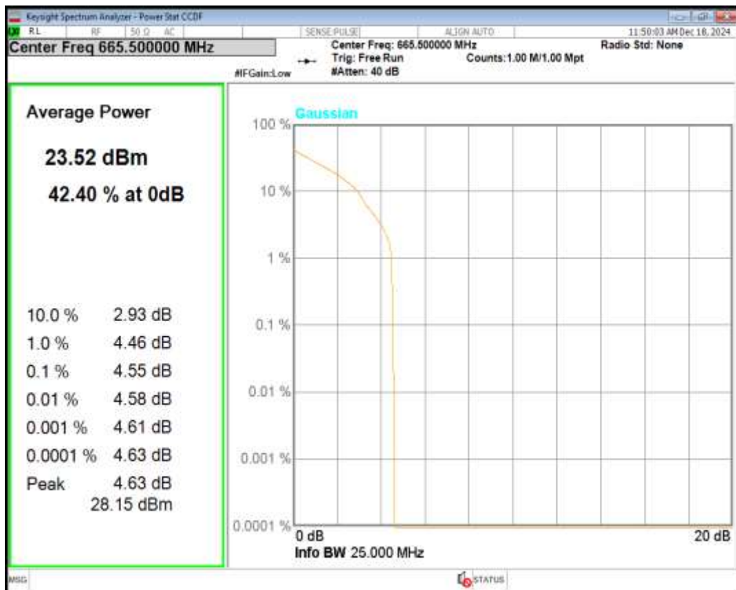
Band71 QPSK BW=5MHz Channel=133297 RB Size=1 Position=#0
