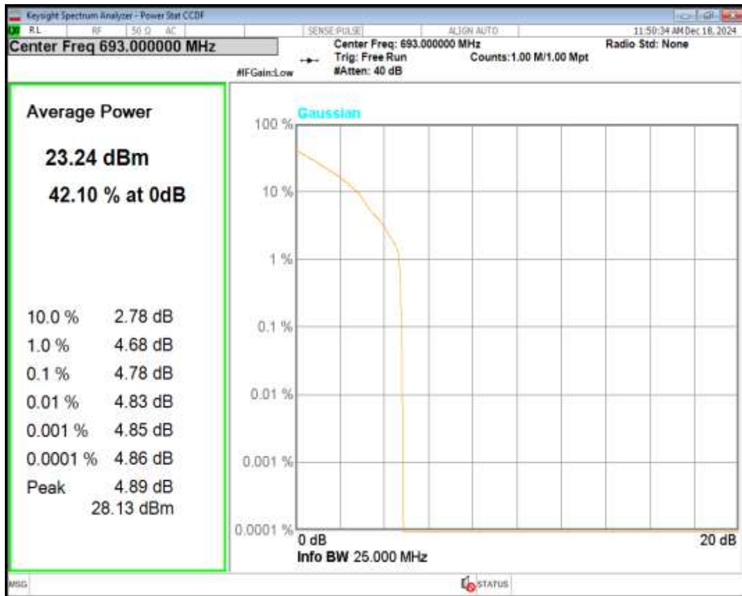
Band71 QPSK BW=15MHz Channel=133197 RB Size=1 Position=#0
