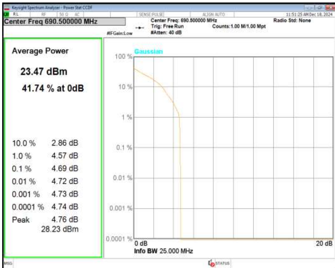
Band71 QPSK BW=20MHz Channel=133222 RB Size=1 Position=#0
