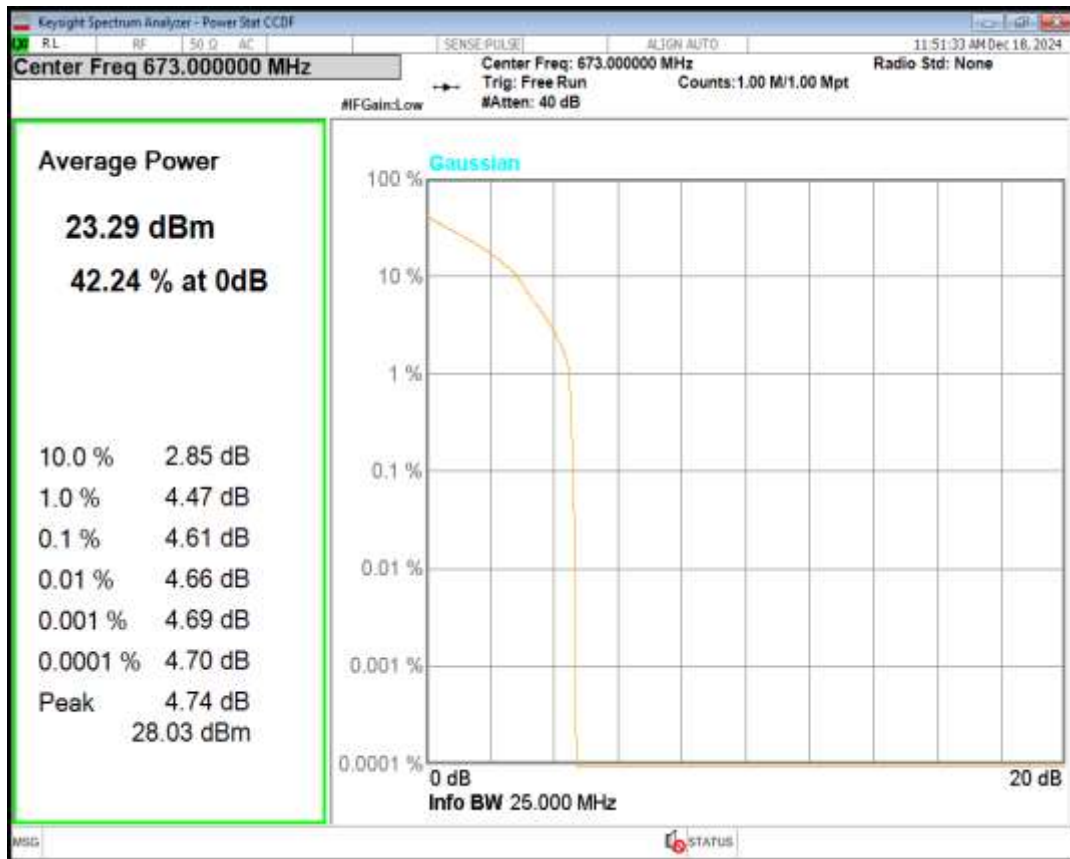
Band71 QPSK BW=20MHz Channel=133297 RB Size=1 Position=#0
