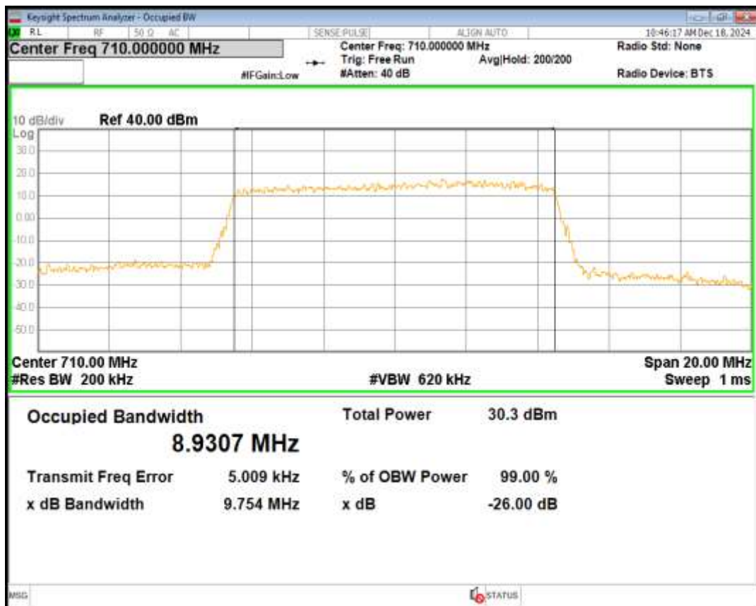
Band17 QPSK BW=10MHz Channel=23800 RB Size=50 Position=#0
