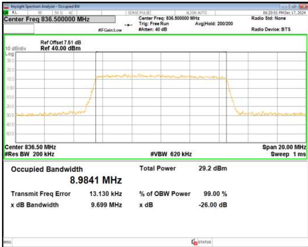
Band5 16QAM BW=10MHz Channel=20600 RB Size=50 Position=#0
