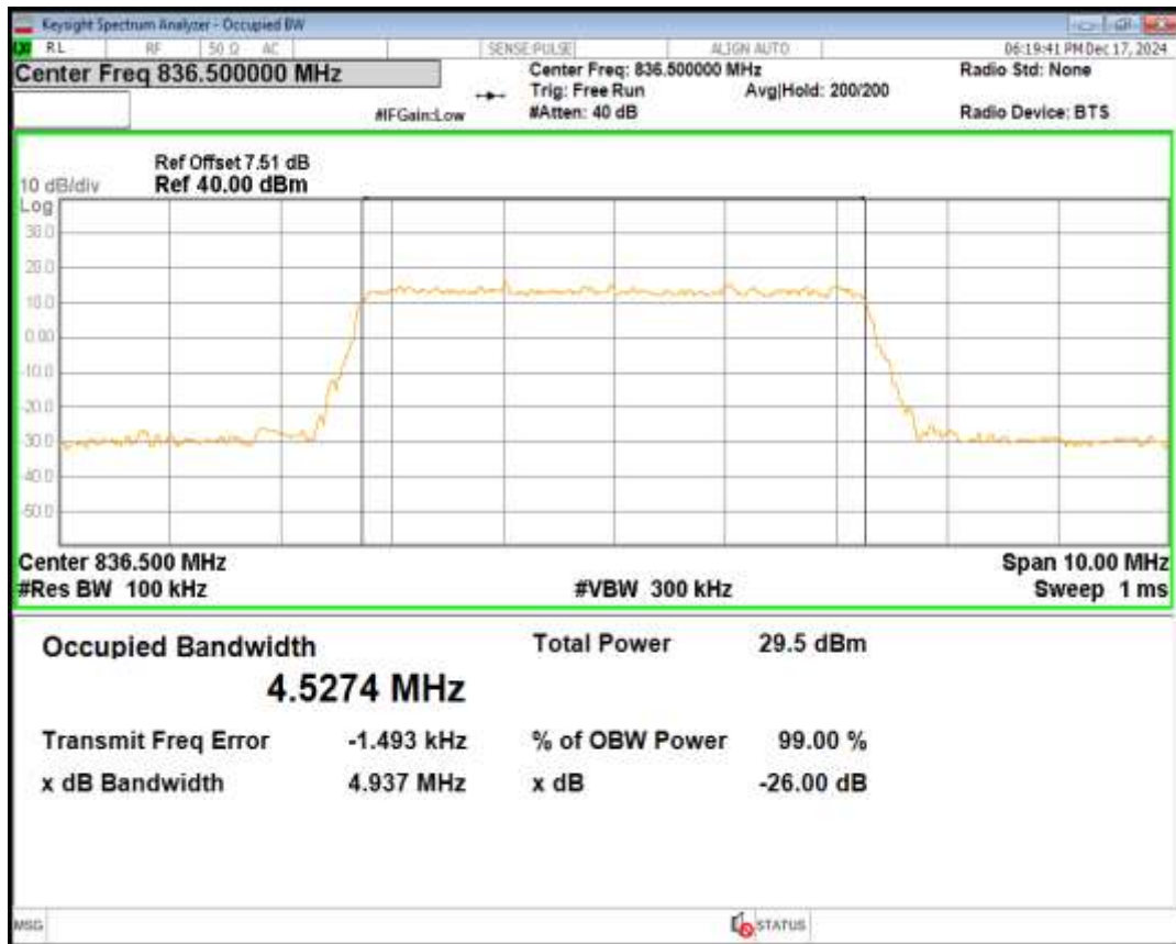
Band5 16QAM BW=5MHz Channel=20425 RB Size=25 Position=#0
