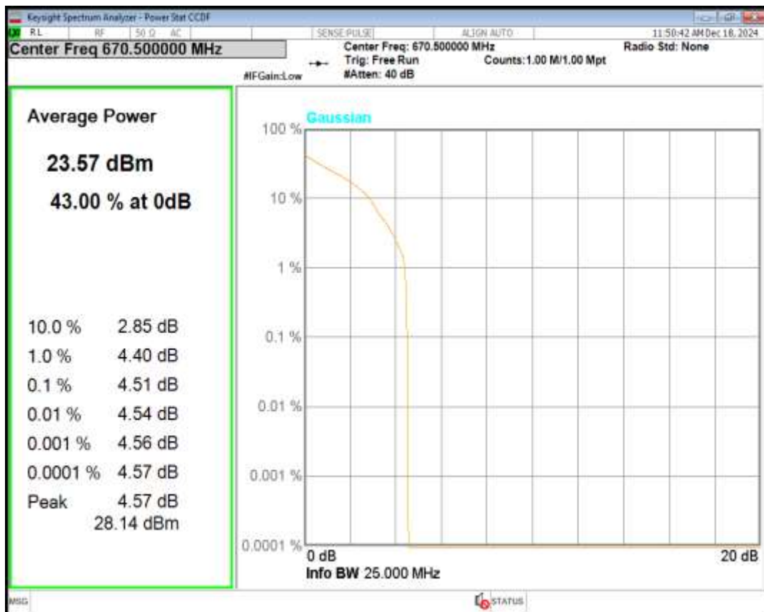
Band71 QPSK BW=15MHz Channel=133297 RB Size=1 Position=#0
