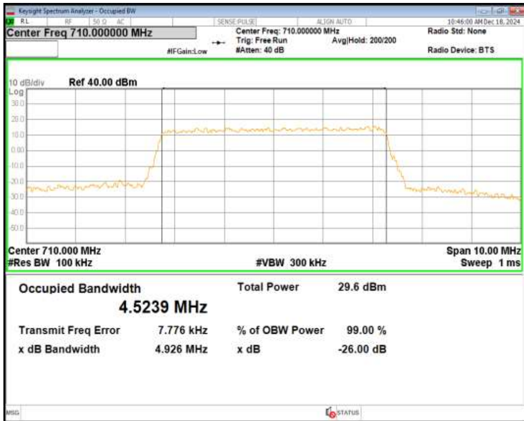
Band17 16QAM BW=5MHz Channel=23825 RB Size=25 Position=#0
