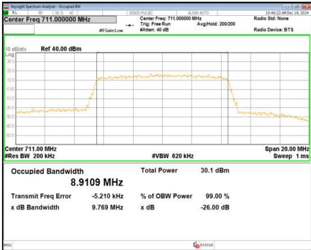
Band17 QPSK BW=5MHz Channel=23755 RB Size=25 Position=#0
