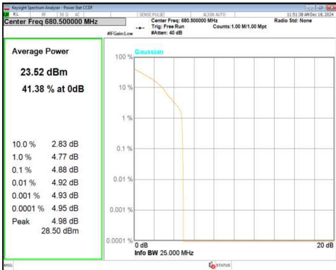
Band71 QPSK BW=20MHz Channel=133372 RB Size=1 Position=#0
