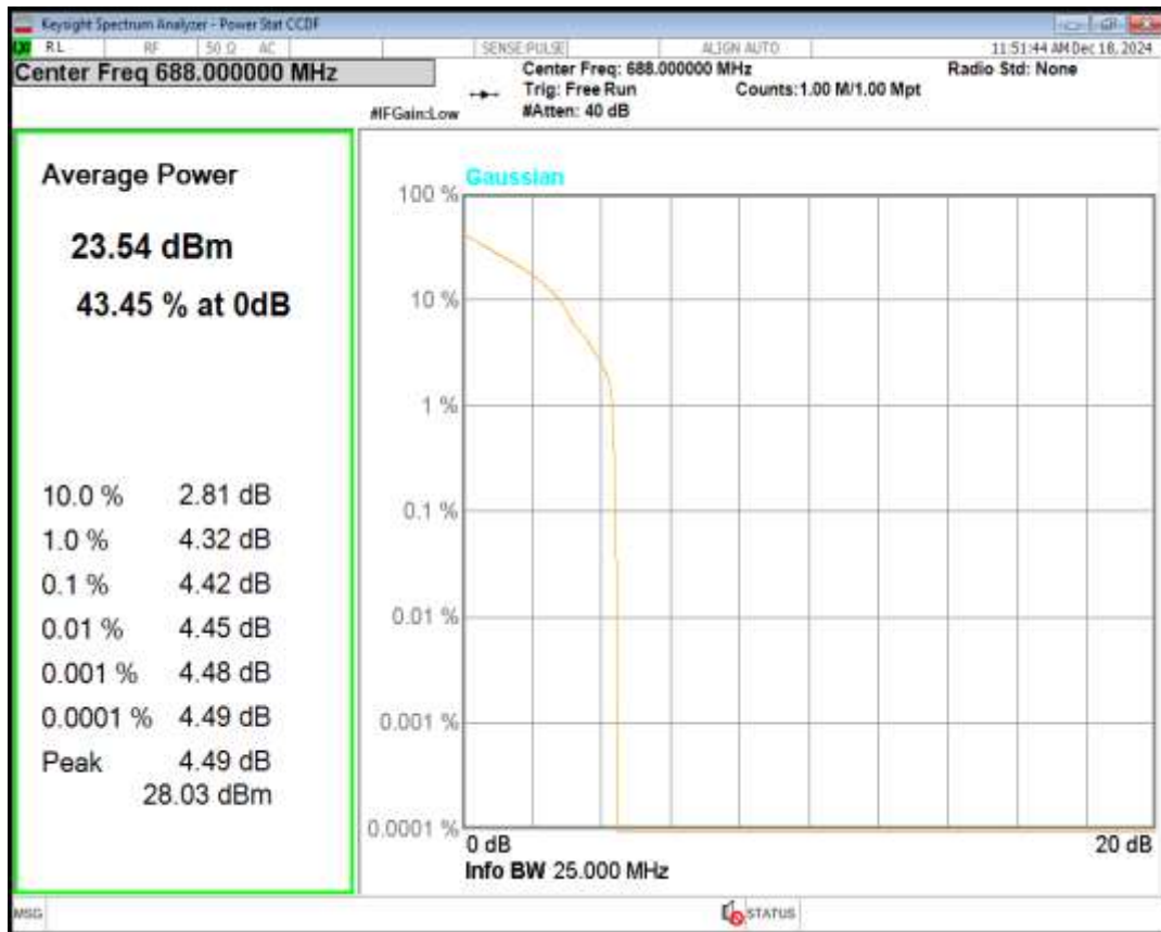
Band71 QPSK BW=5MHz Channel=133147 RB Size=1 Position=#0
