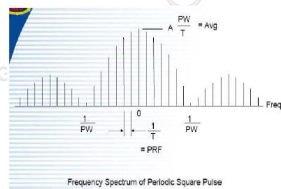
If using spectrum analyzer to measure pulse signal, it have to make sure the RBW use is at least  $2/PW$ .
