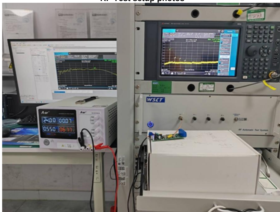
RF Test setup photos
