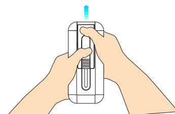
When replacing the batteries, use both hands to remove the back cover of the remote control.
