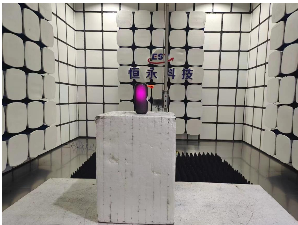
Radiated emission test: Above 1GHz
