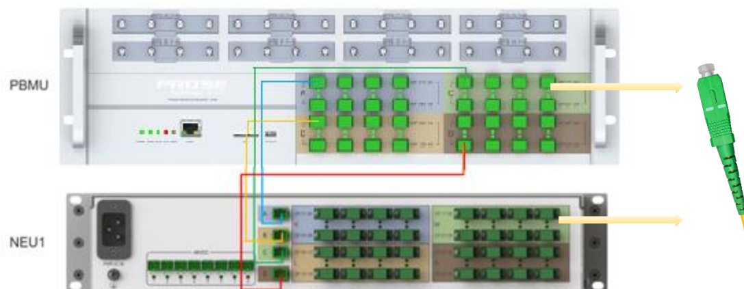
Figure 3-67 Fiber connection between PBMU and NEU
