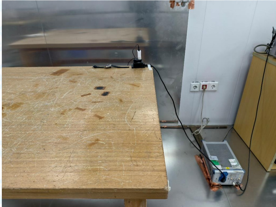
Photo of Setup for Radiated Emission (30MHz~1GHz)
