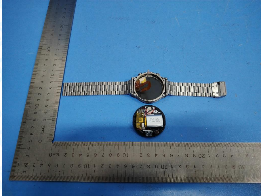
Photo 8 Appearance of PCB & Battery
