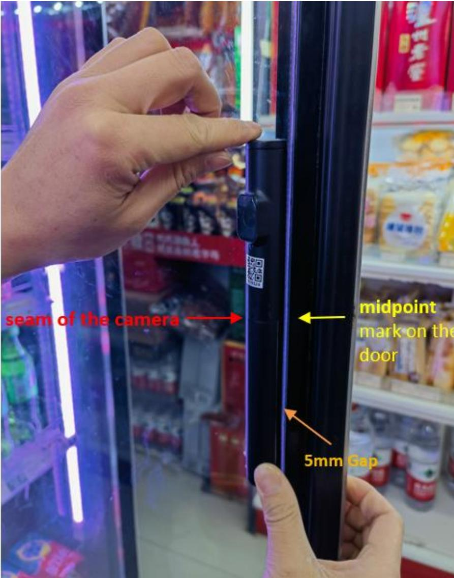
Vertically adhere the camera module to the inner glass.
