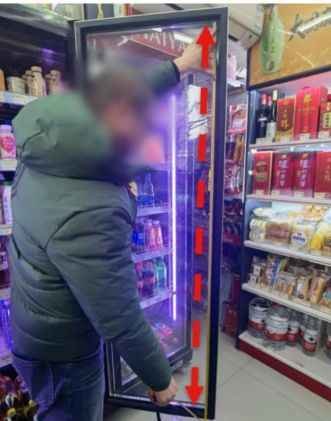
Measure the height of the inner glass of the cooler door.
