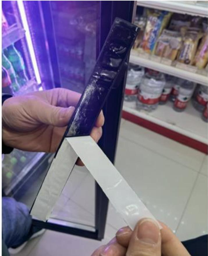
Take out the camera that matches the right-hinged door, and peel off the tape protective film.
