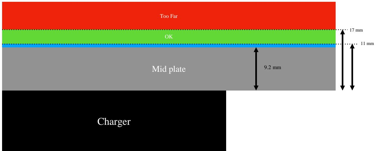
devices. This means that devices must be between 1.8 - 7.8 mm from the mid plate for use in the DCRF.
